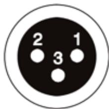
3pins XLR signal output connector (female)
